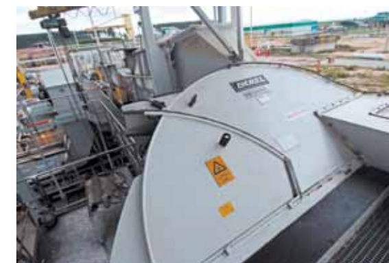
▲ The HHQ-Chipper™, model EXL has a disc diameter of 3.87 m and is equipped with 18 knives.
