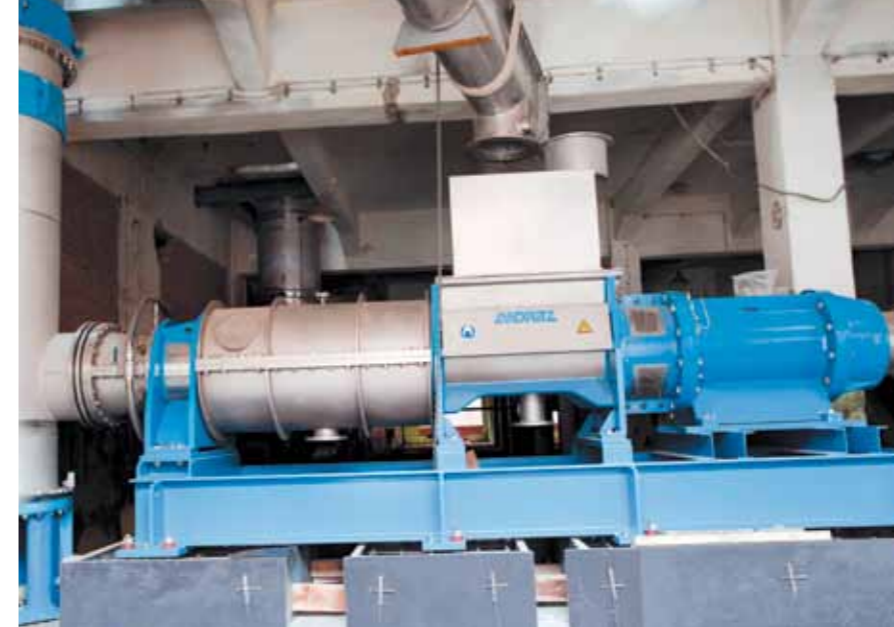
▲ The MSD Impressafiner is a key process step in the P-RC APMP line.
