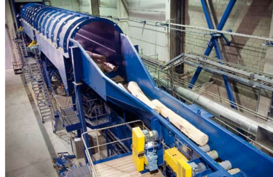
◀ The Andritz RotaBarker™ in the woodyard is a new innovation. It is especially suited for debarking frozen logs in a dry process without costly de-icing. No water is used in the process. Wood losses are minimal.
