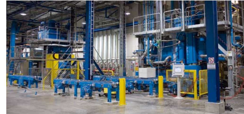
▲ The slab press is the largest in the world. This newly designed unit by Andritz is capable of producing 500 admt/d.
