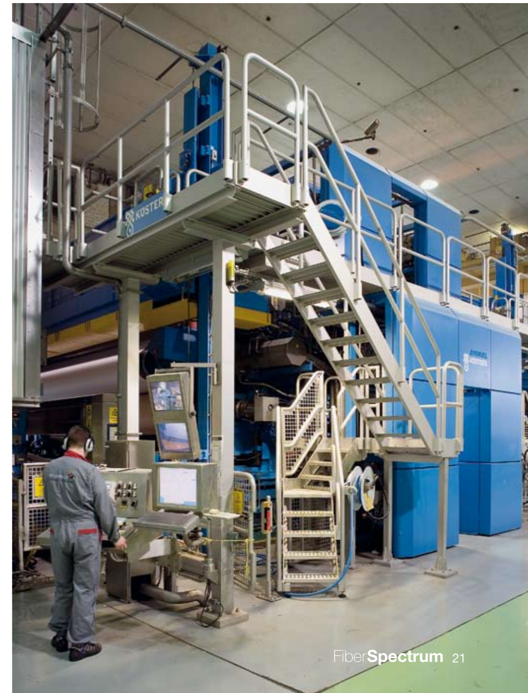
The focus to PM2’s rebuild was the finishing section. ▲ Above: The Andritz Küsters PrimeCal ProSoft calender system consists of two pairs of frames with five rolls each, including PrimeRoll MHV zone-controlled rolls. ▼ Below: An operator checks the profiles on the ProSoft system. Paper widths up to 7.3 m can be calendered at production speeds up to 1600 m/min.
