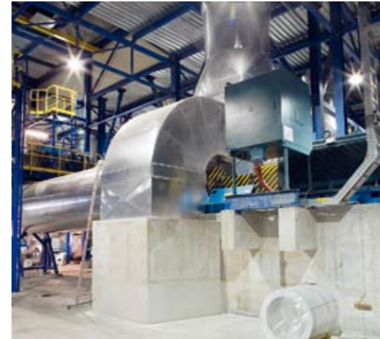
▲ The two-stage flash dryer at Estonian Cell is designed for 500 t/d peak capacity.
