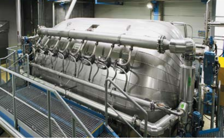
▲ Part of the scope of Andritz's delivery was this CD-Filter which produces excellent white liquor purity.
