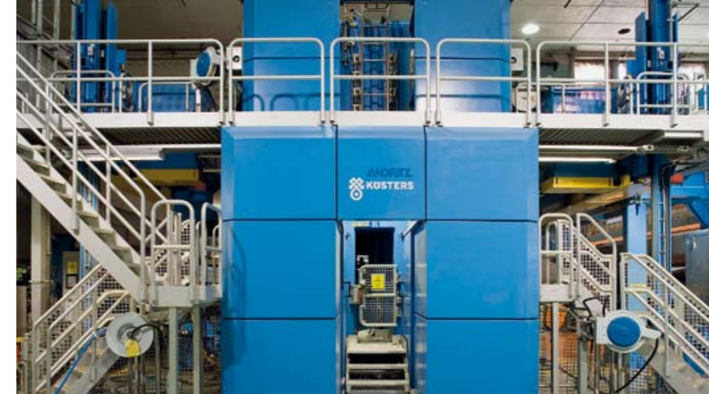
The focus to PM2’s rebuild was the finishing section. ▲ Above: The Andritz Küsters PrimeCal ProSoft calender system consists of two pairs of frames with five rolls each, including PrimeRoll MHV zone-controlled rolls. ▼ Below: An operator checks the profiles on the ProSoft system. Paper widths up to 7.3 m can be calendered at production speeds up to 1600 m/min.
