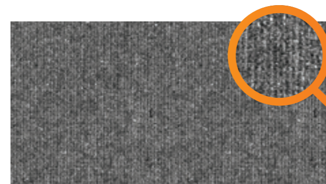
Fig. 7: Conventional fabric design Sample: 15 g/m 2 tissue (pulp + DIP). Speed: 1,750 m/min
