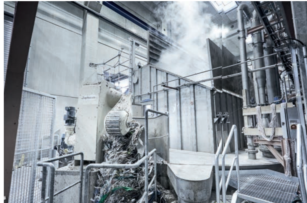
The pulping system with detraging includes a 130 m³ FibreSolve FSR pulper – the largest LC pulper ANDRITZ ever installed in Europe.
