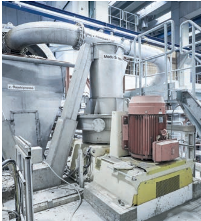
ModuScreens TD tailing screens are part of coarse screening. Efficient washing of fibers is done with a FibreWash Drum – one important part of the detraging system.
