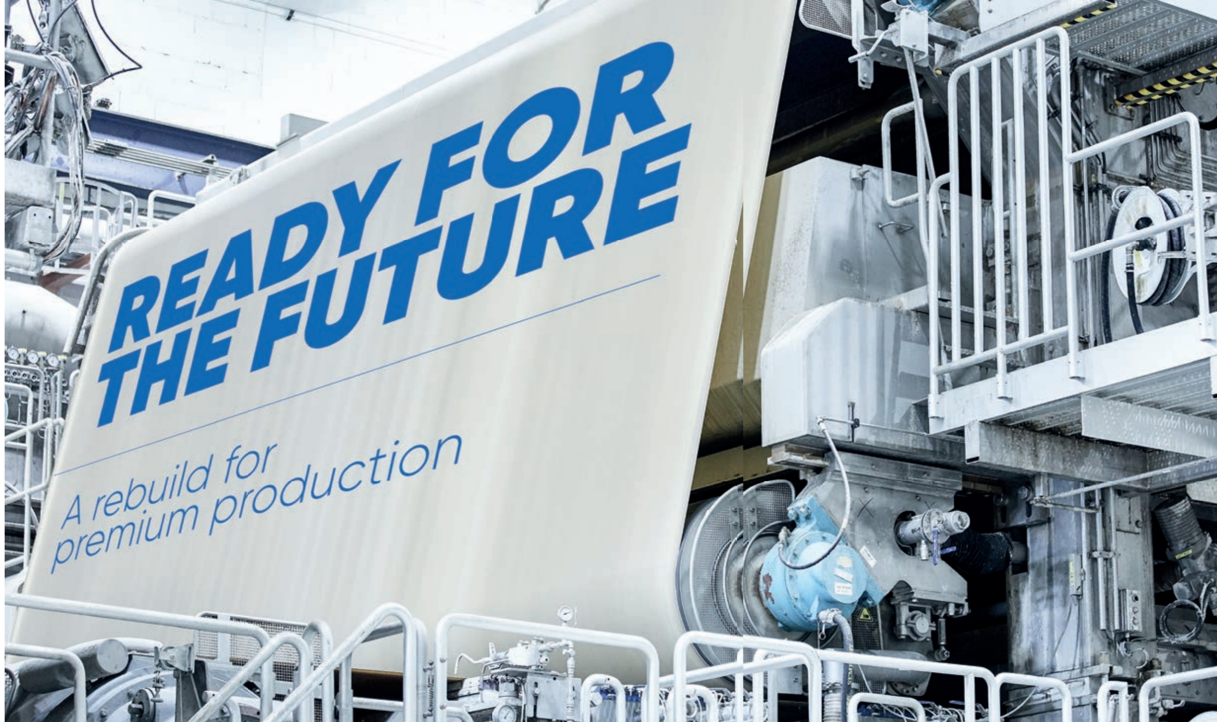
PrimeDry Steel cylinders yield better drying performance with the same size and operating pressure as traditional cast-iron cylinders, and thus help to increase production or save energy.
